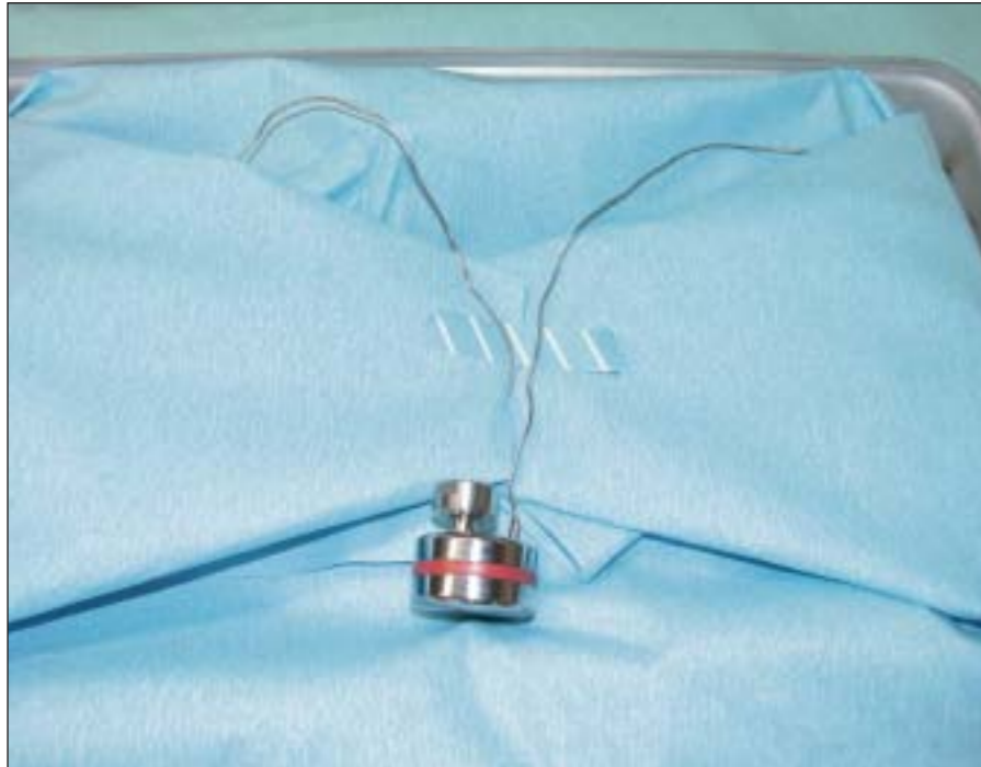
Pressure-temperature data logger EBI-125 A PD3 with flexible temperature sensors, diameter < 2mm.
