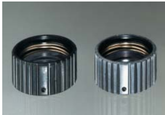
Aluminium corrosion after 100 runs of a chemothermal Programmes at 60 °C. Left: with mildly alkaline cleaner in softened water. Right: no addition, softened water alone.
